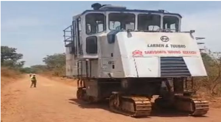
Image 6: Surface Miner Arriving on Site
