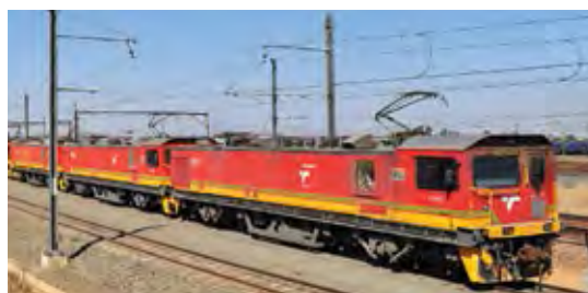
Dual-voltage class 19E locomotives, built between 2007 and 2011. Photo: Eugene Armer.
