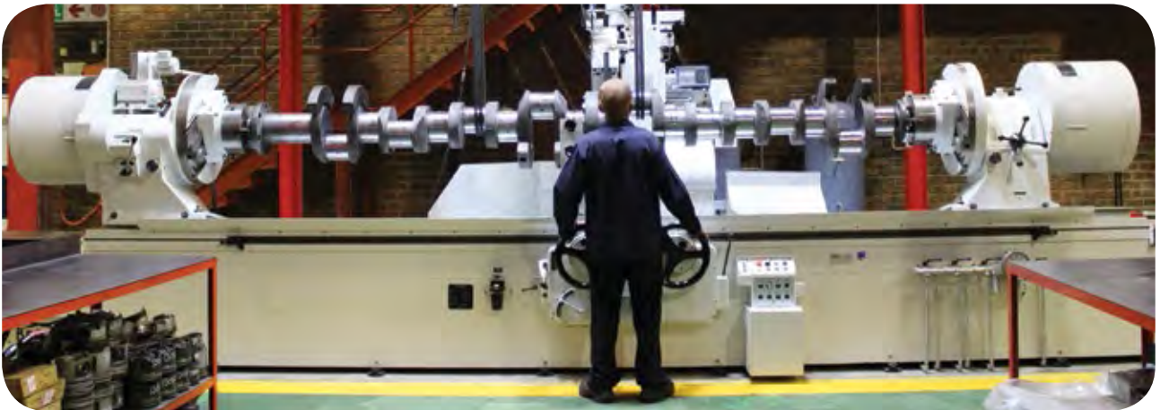
Grinding of crankshafts with lengths of up to 4.7 metres and weights of up to 5 ton
