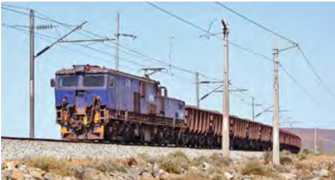
A class 9E (50kV AC) electric banking behind an export iron ore train to Saldanha. Photo: Joyce van der Vyver.
