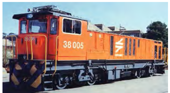
UCW built these class 38 electro-diesels in 1990, able to work under 3kV DC catenary, or away from the wires.
