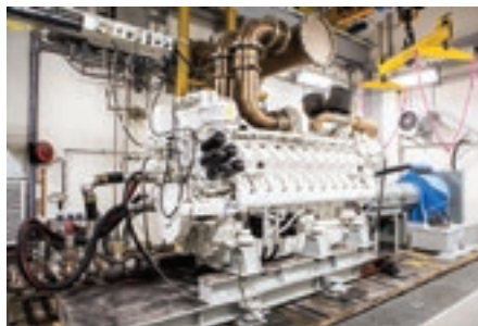
Upgraded test bench with a Series 4000.
