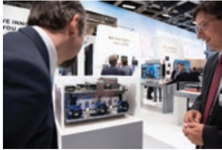
MITRAC converter Module P offers up to 45% less volume and up to 35% less weight compared to other converters for metro applications of the same performance class.
