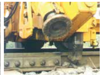
Figure 4: Specialised lifting and aligning unit found on universal tamping machines.
