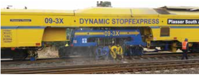
Figure 16: The tamping units are mounted to a separate frame on continuous action tamping machines.
