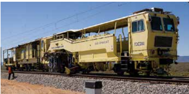
Figure 17: DYNA-CAT Universal tamping machine.
