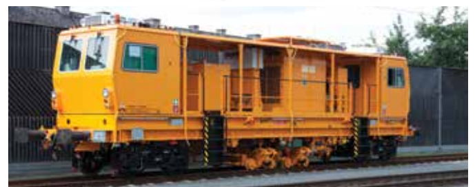
Figure 19: Stabilising units located between the bogies.
