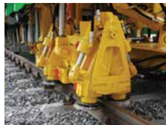
Figure 3: A typical lifting and aligning unit found on plain track tamping machines.
