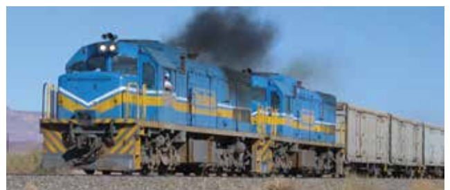
TransNamib freight train behind former South African class 33 (GE U20C) locos, dating from the late 1960s. Photo Harald Süpflé.
