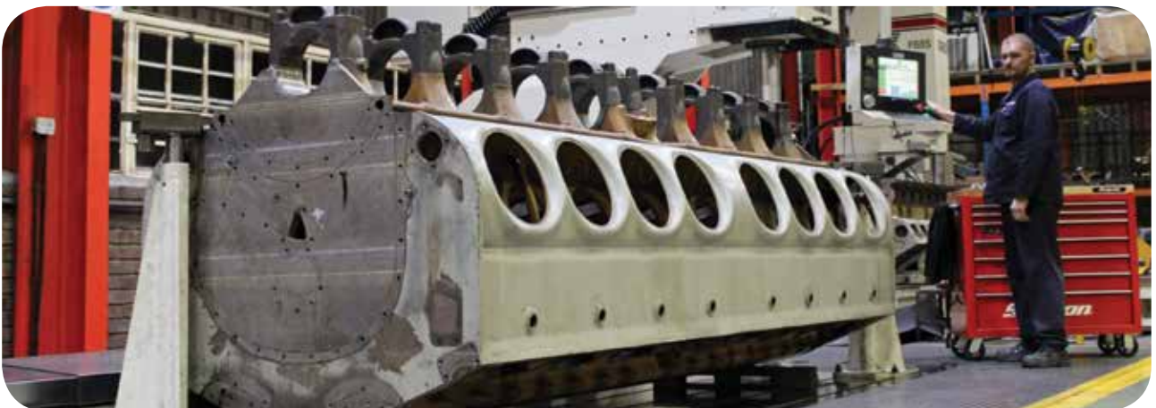
Lineboring, boring, milling, 3-axis machining and blue printing of blocks over 6 metres
