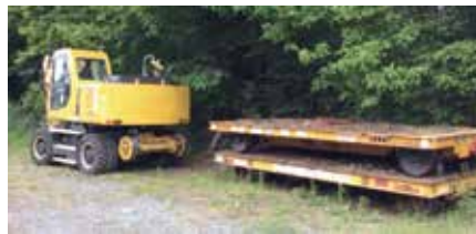
The road rail vehicle and trailers used to collect scrap sleepers. Photo: Network Rail.
