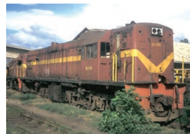
Ex-South African 1,975hp class 32 loco photographed in the DRC by Martin Welzel in 1991. GE U18C1 type, 1-Co-Co-1, dating from 1959.
