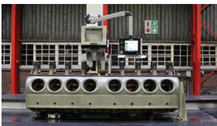
The CNC machining centre is capable of lineboring, surfacing and blue-printing blocks over six metres in length.
