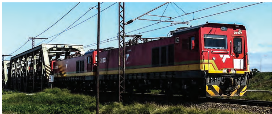
Chinese-built class 20E electric locos crossing the Swartkops River at Port Elizabeth with a manganese consist. Photo: Richard Gillatt.
